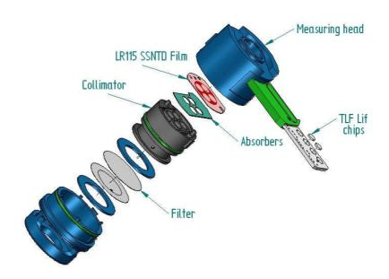
A solid state nuclear trace detector (cellulose nitrate LR115) ahead, facing the sampling filter, collects the alpha emissions of short-lived radon 222 and 220 isotopes.
