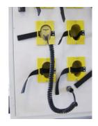
Mass flowmeter: measures the sampling flow rate of each dosimeter.
