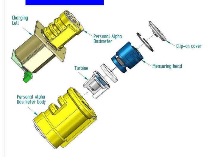
A battery powered centrifugal turbine ensures a flow rate adapted to the aeraulic properties of the measuring head.
