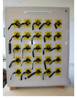
**Charge regulator:** checks and adjusts the charge current supplied by the charging dock to the sampler's battery.
