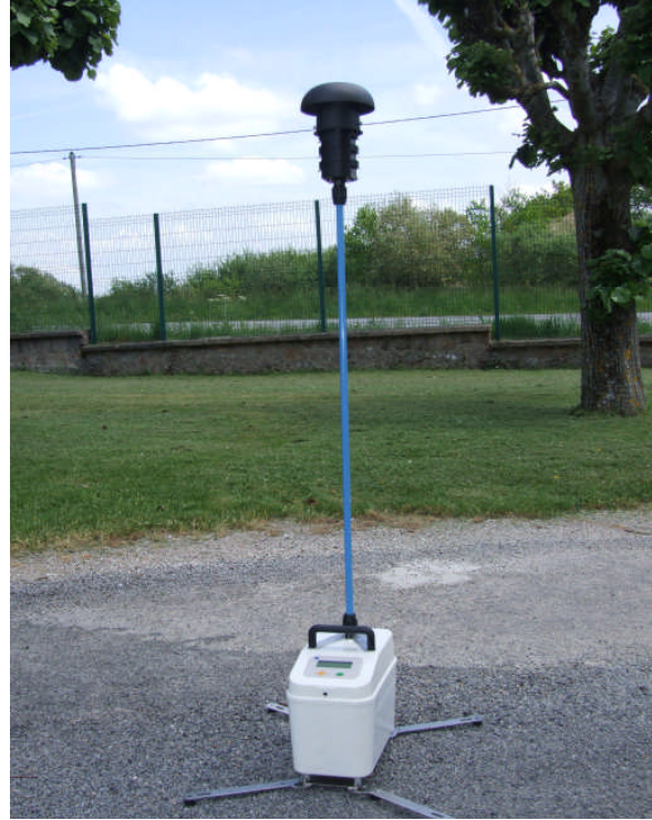
PA1000Gamma with sampling head, elevating kit and stabilisers
